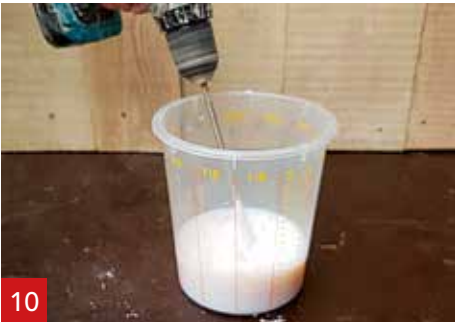
Put the mixer (skew) in the A1 Liquid cup and create a swirl.
