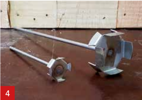
Use the A1 mixer. Small: up to 1.5 kg of A1. Large: 1.5 kg or more A1.
