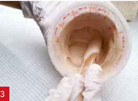
3 Mix the A1 Liquid, Thix A and A1 Powder resulting in a smooth material.
