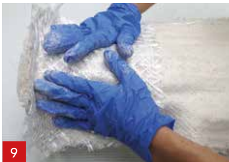
6 Add the A1 Triaxial fibre on the wet A1. Continue until the entire silicone mould is covered with A1 and a layer of A1 Triaxial fibre.
