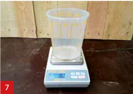
Place a cup on the scale. Calibrate the scale together with the cup (0.0 g).
