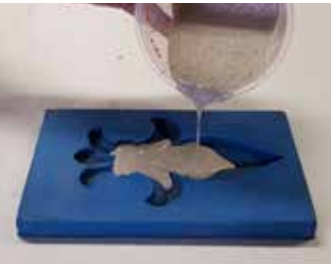
Pour part of the created A1 into the mould. Start (if possible) by brushing the mould, so that all unevenness/relief is touched with A1.
