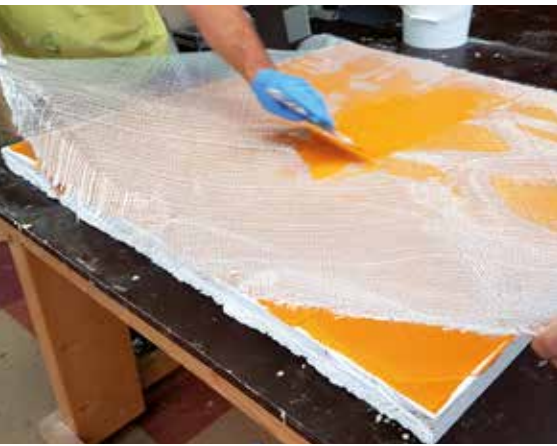
Before applying the A1 Triaxial fibre, cut it to size first, given the processing time of A1.
