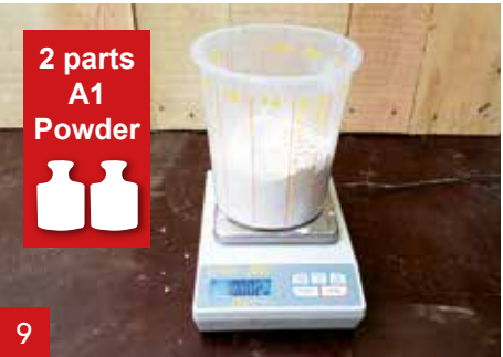
Weigh 2 parts of A1 Powder. In this example we use 1000 g A1 Powder.
