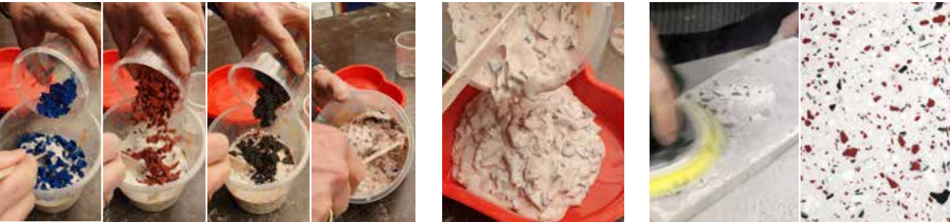
Add different colours of broken A1 to the mixed A1 and stir well.
