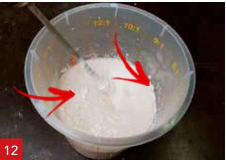
Stir the mixer till all lumps have disappeared (± 1 min.) resulting in a smooth material.
