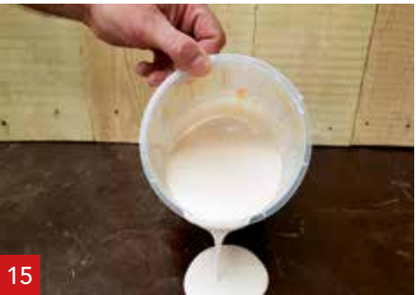
A1 is ready for laminating, casting or spraying. Processing time 20 - 25 minutes.
