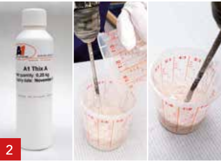
2 Add 2% Thix A (of the total quantity A1) to the A1 Liquid. By using Thix A the A1 will result in a thicker texture.
